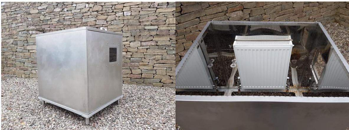
Following requests from many interested parties who wished to see Blueproof in action, the team devised this portable functional test oven to show exactly how the fire suppression device is triggered in the case of fire.
